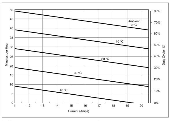
Figure 1. Allowable Duration of Current >11 A
