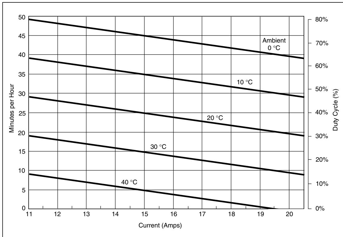
**Figure 1. Allowable Duration of Current >11 A****Resistance**
